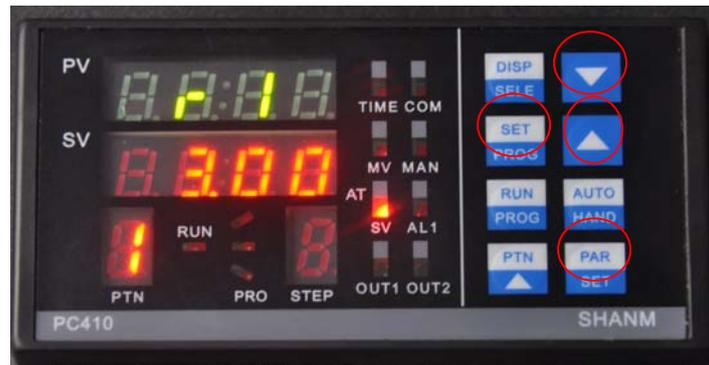
3) L1 means the first seted temoweature, press
