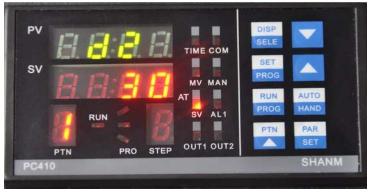
8) r3 means the 3<sup>rd</sup>, temperature rate, we set 3.00, then press
