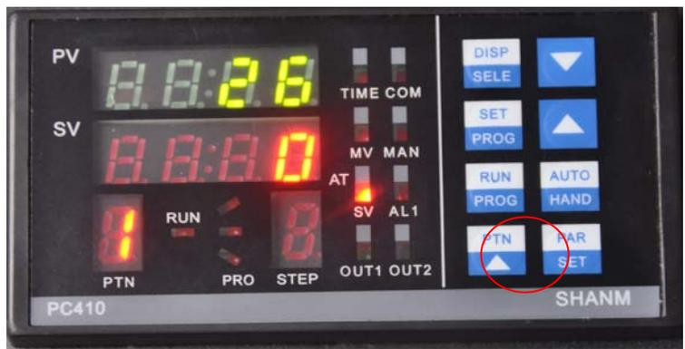
2) press **SET** **PROG** key to set the curve, r1 means the first temperature rate, 3.00 means Heating up 3 degrees per second
