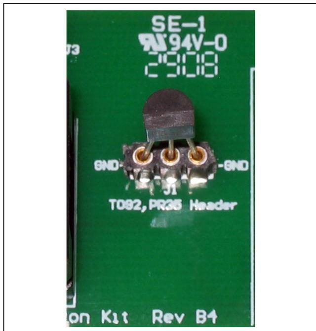
Figure 3. TO92/PR35 Package Insertion
