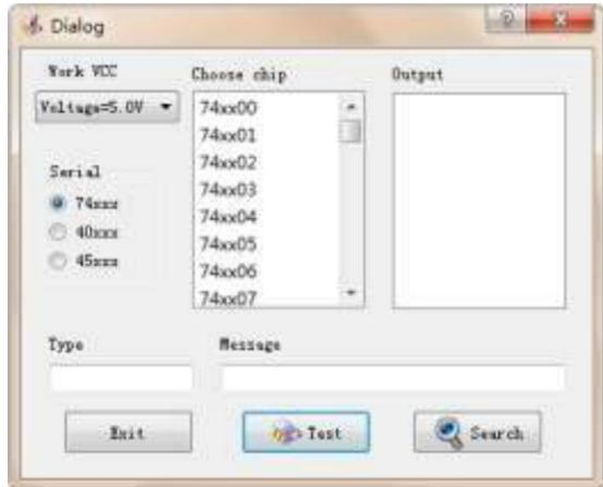
Choose the series type under test device, model after press test. If the device is good,
